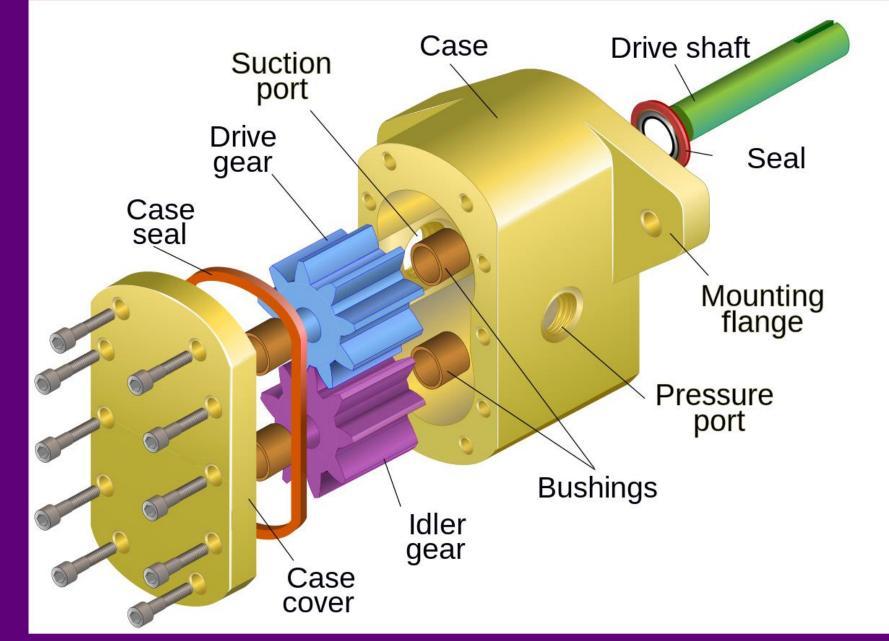
An exploded view of an external gear pump by <u>Duk</u>, vectorised by <u>Д.Ильин</u> and made multilingual by <u>cmglee</u>. https://creativecommons.org/licenses/by-sa/4.0/ https://commons.wikimedia.org/wiki/File:Gear\_pump\_exploded.svg
